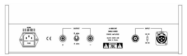
Figure 4 - A-5000 DHT Rear Panel View
